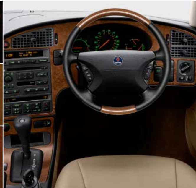
Wood and leather steering wheel – with genuine cultivated mahogany inserts in light or red nuance. Partly leather-trimmed for safer grip. Accepts the airbag module and audio control buttons from the car's existing steering wheel. Must be fitted according to Saab technical standards to ensure airbag functionality. Saab 9-5 until model year 2005.
