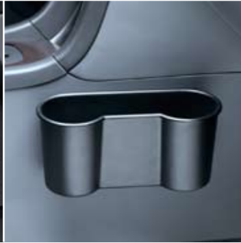
Waste/storage box – fitted on the passenger side of the centre console. Designed as a holder for two soft-drink cans. Five CD discs can be stored in the middle section. Can alternatively be used to hold a waste bag.
