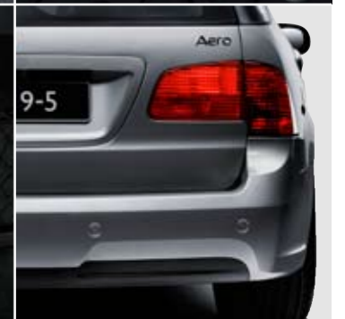
Saab Park Assist (SPA) – makes it easier to judge rear distances when parking in tight spots. SPA automatically detects and adjusts the activation range if the car is equipped with a towbar. SPA is also automatically switched off when a trailer is hooked up.
