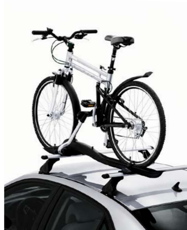
Bike holder – for mounting on the roof rack. Can be adjusted to accommodate a variety of bikes. The bike is secured in an upright position. Unique latching feature makes it easy to secure the bike. Lockable. Made of fibreglass-reinforced polyamide.
